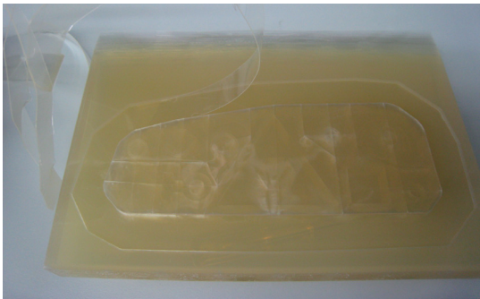
Fig. 11. Waste-material removal in LOM
