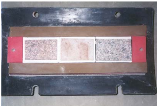
Fig. 2. Three rock plates installed on the inside part of the top of the mill (from [5])
